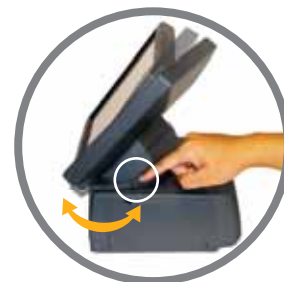
Ergonomic design allows LCD display swivel angle 0° to 16° in clockwise direction for improved viewing angles
